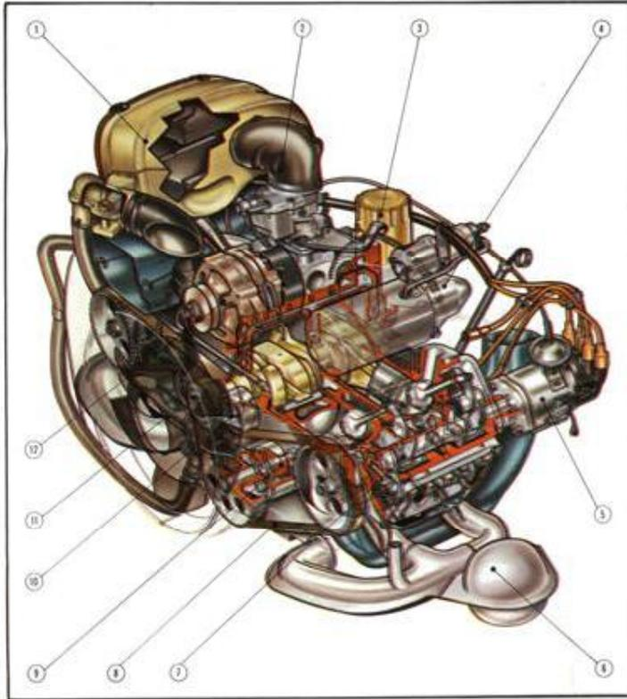
At launch, in October 1970, the carburettor hotspot was heated by engine oil, but this gave problems with slow warm-up, so a revised heating arrangement using exhaust gas was used. This lasted throughout the life of the engine, though it made one of the most complicated exhaust systems around - 12 different pipes and 9 clamps of 4 different types.
