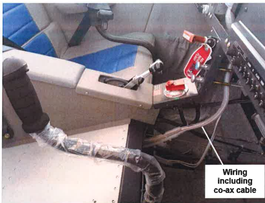
Figure 15 Dismantling of the right side panel from the middle channel under the instrument panel
